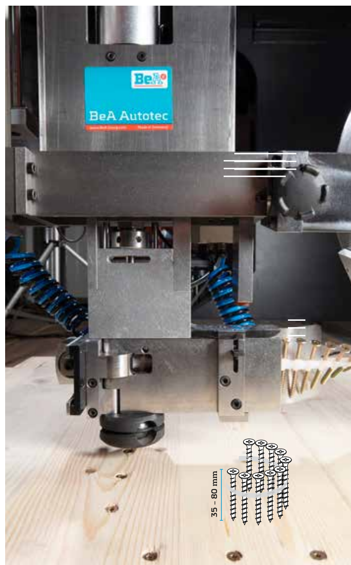
Jumbo coil: Magazine capacity 700 Screws
